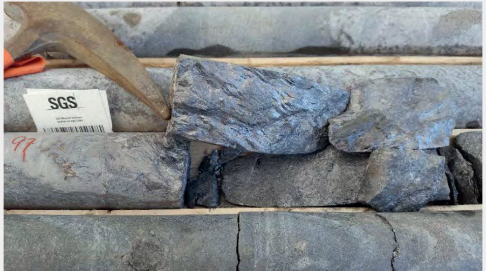
High-grade vein graphite in drill core from Buckingham. ( Source )
