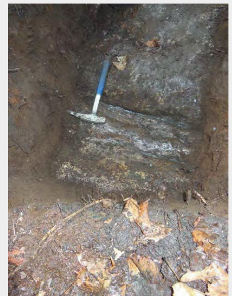
Graphite mineralization in a 0.5 m pit on a strong beep mat anomaly at Buckingham (Robillard, 2013; Source )
