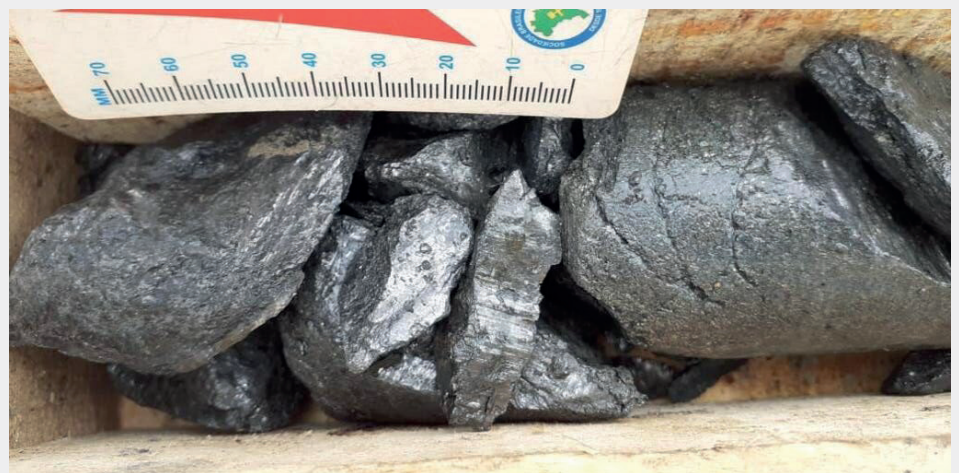
Core from Gratomic’s maiden drill program at Capim Grosso, showing high-grade graphite.
