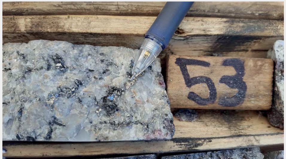
Large flakes of graphite in drill core from Buckingham. ( Source )
